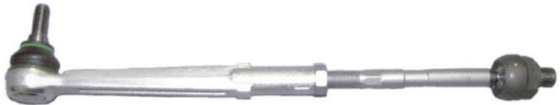
Hybrid Aluminium - Stahl Design Porsche 911 & Boxster
